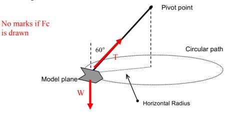
(a) On the diagram above, draw the forces acting on the model plane
