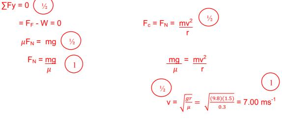
(b) Calculate the minimum revolution rate in rpm the disc must spin at for the block not to slip and fall. (if you could not answer (a), use  $v = 3.50 \text{ ms}^{-1}$ )
